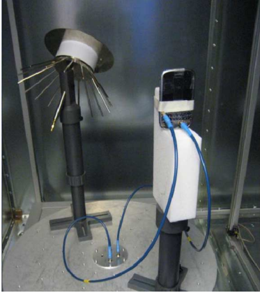
Fig. 12. The two branch antenna was measured in a RC for diversity gain and capacity measurement.
