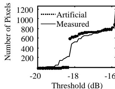
Figure 1: Metric comparison for representative artificial and measured image pair
