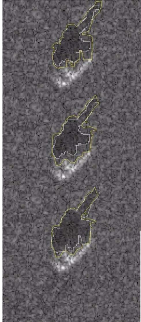
Figure 8: Manual and automatic segmentation of test shadow. Top two sections compare automatic with two different manual segmentations, bottom section compares the two manual segmentations.
